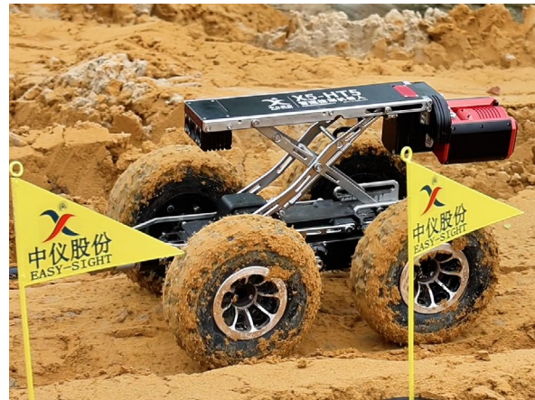
the X5-HT5 pipeline measurement robot
